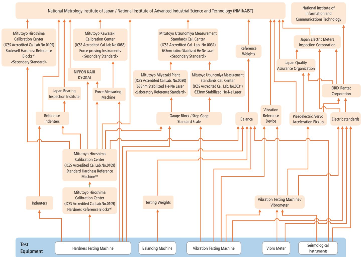
\*1 The scope of JCSS accreditation is from 20HRC up to 65HRC in Rockwell Hardness Testing Machines and Hardness Reference Blocks.
